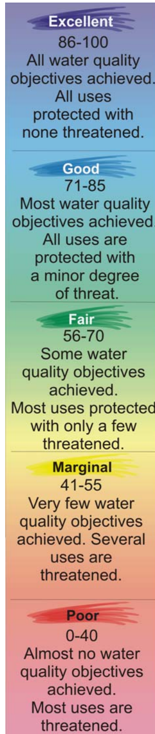
Figure 5. Scale used for Alberta Agriculture Water Quality Index (Courtesy Sarah Depoe, AAFRD)
